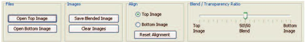
This toolbar opens the Image Comparison window and loads the selected image into either the top or bottom slot for variable opacity image blending and comparison.
